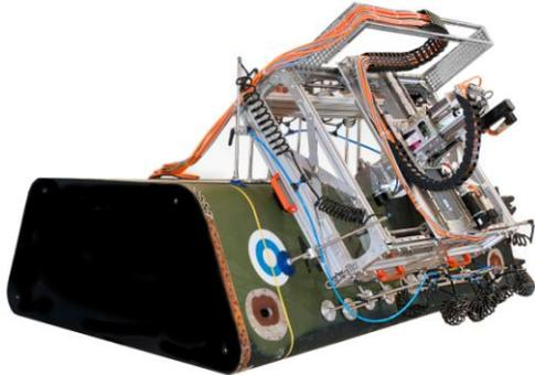
Fig. 5: Prototype mobile milling machine (photo © WIWeB, Primacon)
