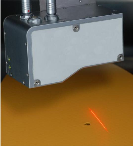
*Fig. 1: Machine-integrated line scanning of composite components*
