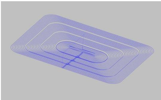
Fig. 2: Nominal NC path for a rectangular patch
