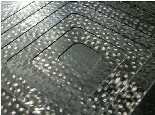
Fig. 6: Stepped scarfing (photo © WIWeB, Hufschmied)
